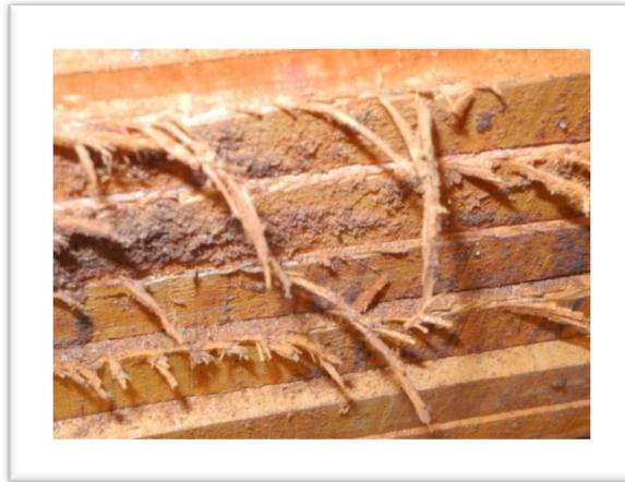
Photo (6): Engine RPM too low may result filamentous timber
