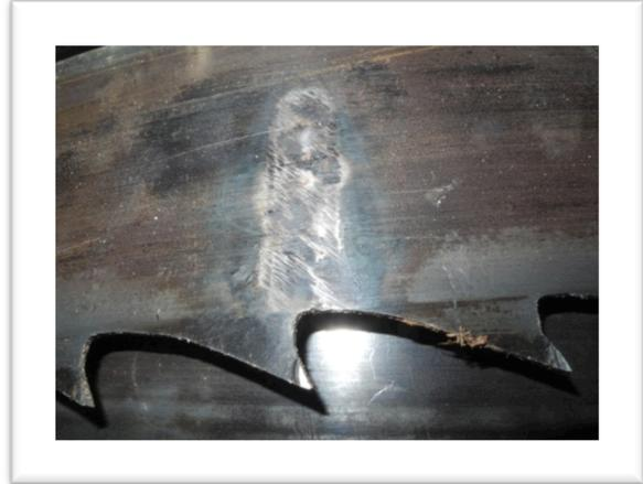
Photo (5): saw blade and gullet shape does not fit
